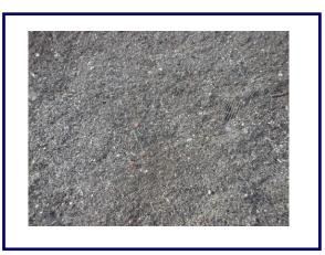
DESCRIPTION: Fresh production; originating from the machining of cast-iron and
